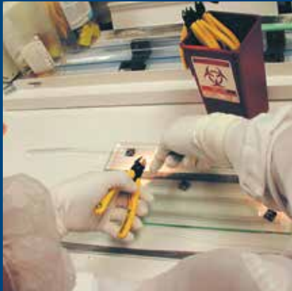
Technician cuts catheter wire to length using 80 Series 8150 cutter.
