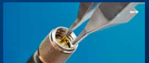
7292MI micro-mini end cutter is used to cut wire inside a mini connector.
